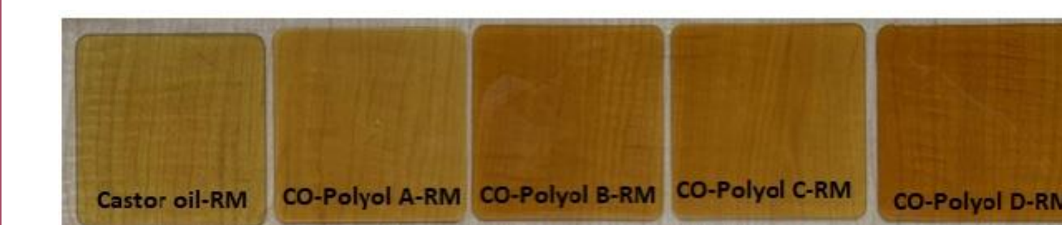
Fig. 7 Elastomers prepared from castor oil and self condensed castor oil
