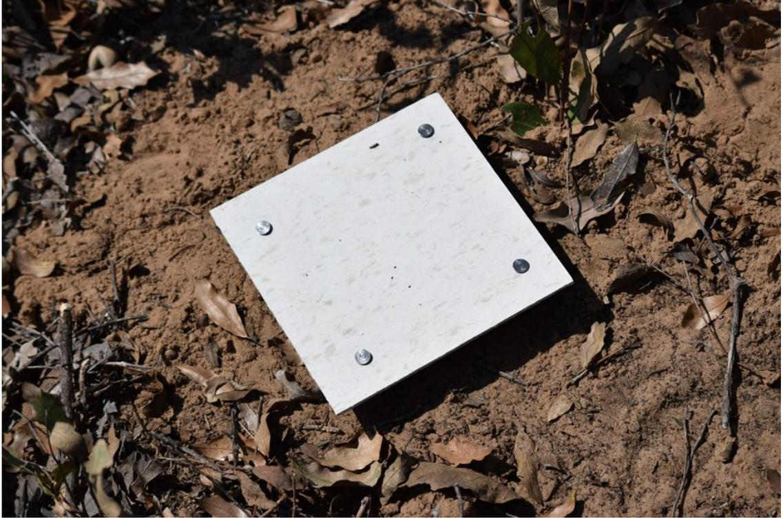
Figure 6. A deployed and covered pitfall trap in shinnery oak habitat. The cover was made from a lineolium floor tile, its purpose being to reduce evaporation of the preservative by providing shade and discourage entry by small vertebrates.
