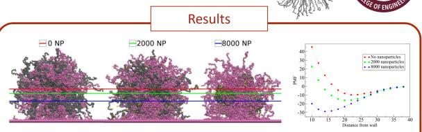
The equilibrium distance between colloid and wall decreases as the number of sticky nanoparticles in the system increases. Horizontal lines show the location of the center of the colloid sphere for systems with 0, 2000 and 8000 sticky nanoparticles. (Nanoparticles not shown.) PMF of the colloid center of mass coordinate as a function of distance from the wall for these three systems.
