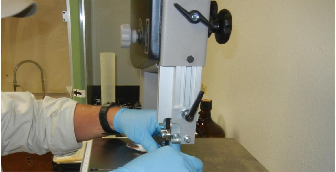
**Figure 26:** Crabs were cut along the medial line using a band saw.
