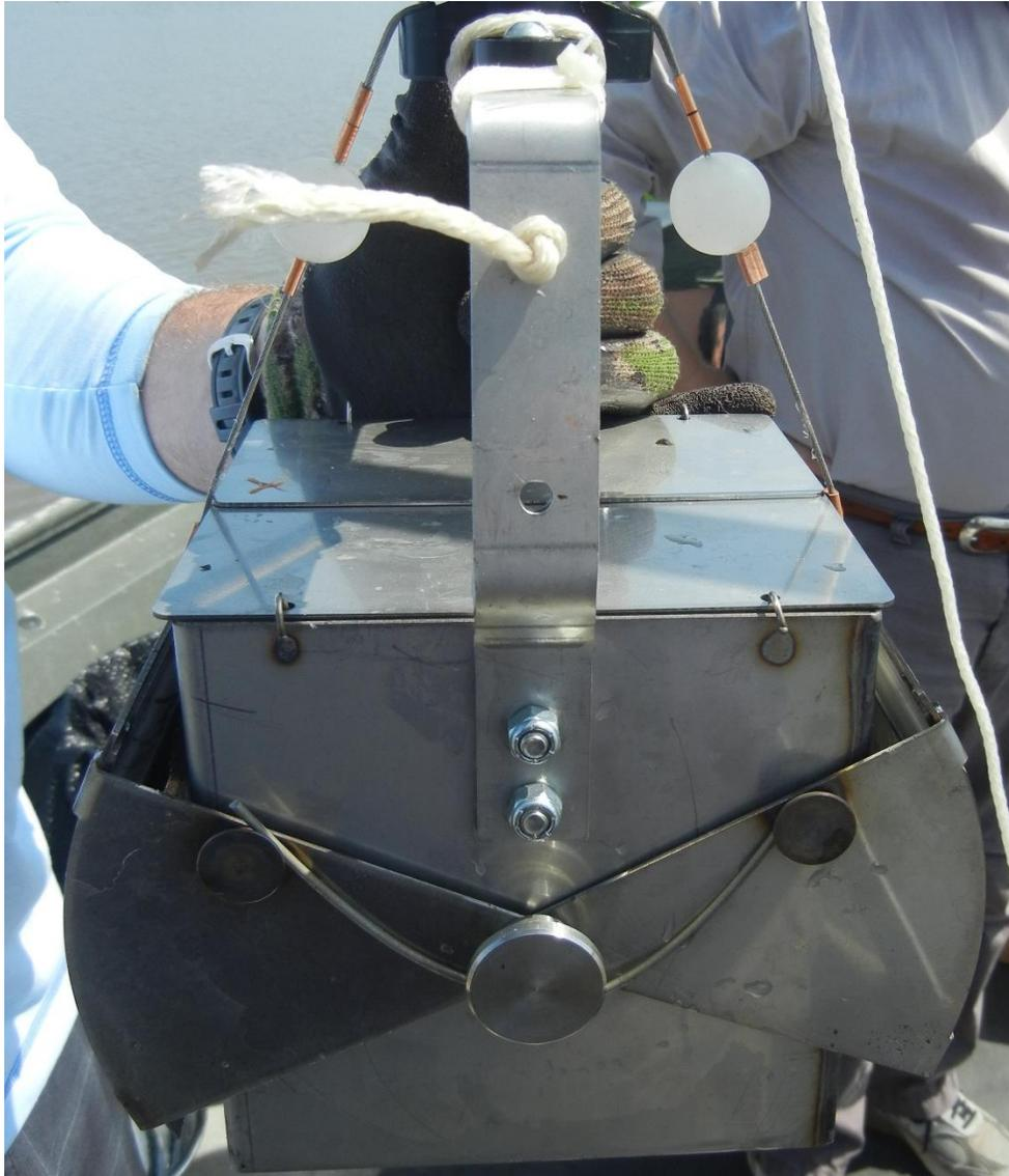
**Figure 18:** Ekman bottom grab sampler from Rickly Hydrological Corporation.
