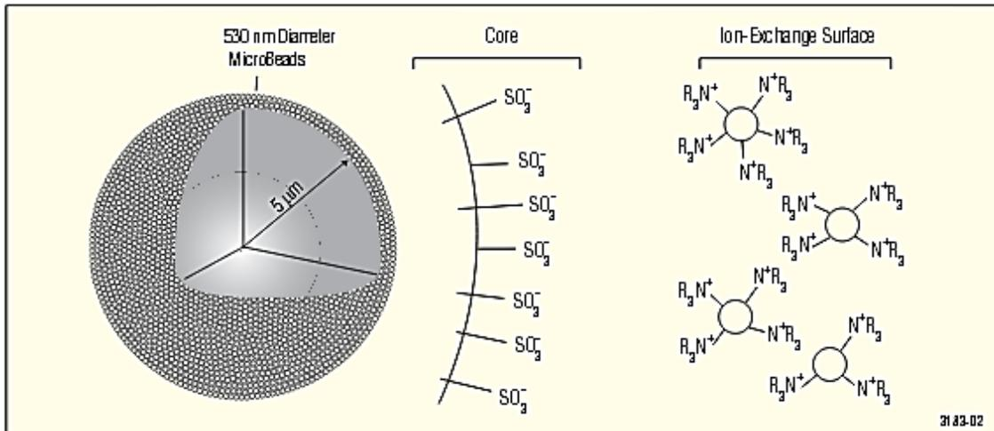
**Figure 36:** IonPac™ AS7 anion exchange column packing (Dionex Corporation, 2006).
