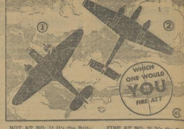
NOT AT NO. 1! It's the British Blenheim, a mid-wing medium bomber, powered by twinradical engines. The nose of the fuselage extends forward of the engine nacelles. The wings taper almost equally to rounded tips. The tips of the tailplane are also rounded and it has a single fin and rudder.
