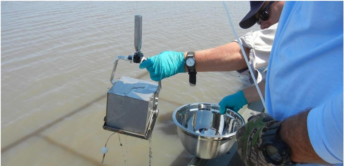
**Figure 20:** Ekman sampler being pulled from location L-1 in East White Lake.
