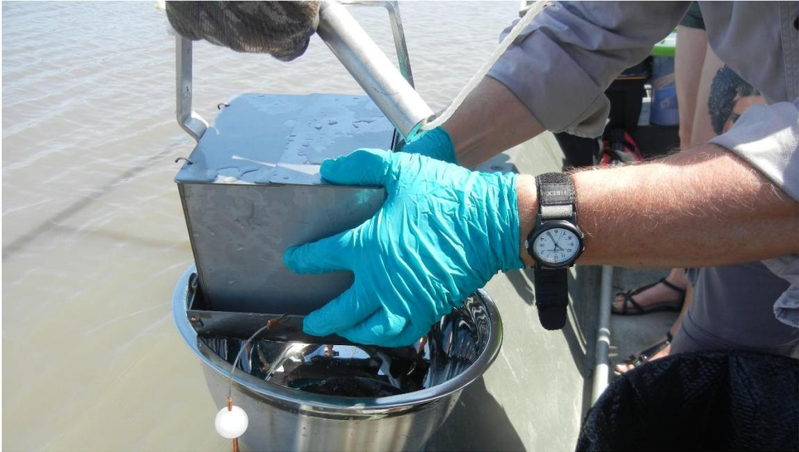
**Figure 21:** Emptying sediment from the Ekman sampler at location L-1 into a clean stainless steel bowl.
