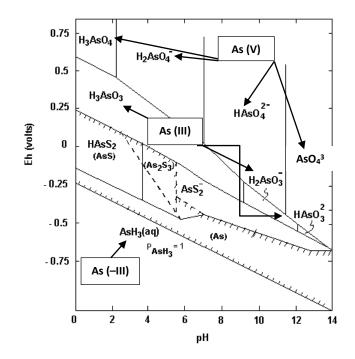
**Figure 1**: The  $E_{H}$ –pH diagram for As at 25°C and one atmosphere with total arsenic 10<sup>-5</sup> mol/L and total sulfur 10<sup>-3</sup> mol/L. Solid species are enclosed in parentheses in cross–hatched area, which indicates solubility less than 10<sup>-5.3</sup> mol/L. Reproduced from Ferguson and Gavis (1972) with permission from Elsevier.
