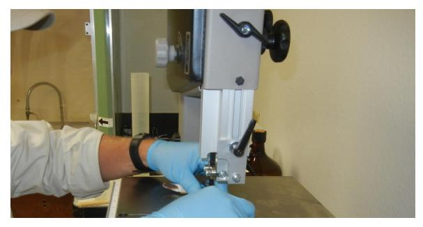
Figure 26: Crabs were cut along the medial line using a band saw.
