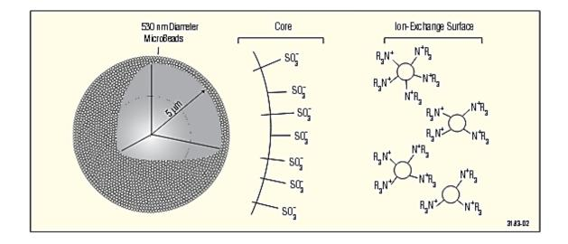
Figure 36: IonPac<sup>™</sup> AS7 anion exchange column packing (Dionex Corporation, 2006).
