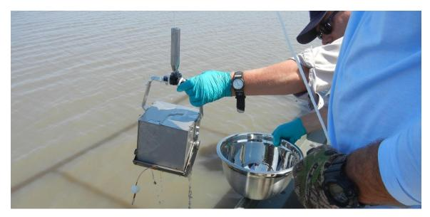
**Figure 20**: Ekman sampler being pulled from location L–1 in East White Lake.
