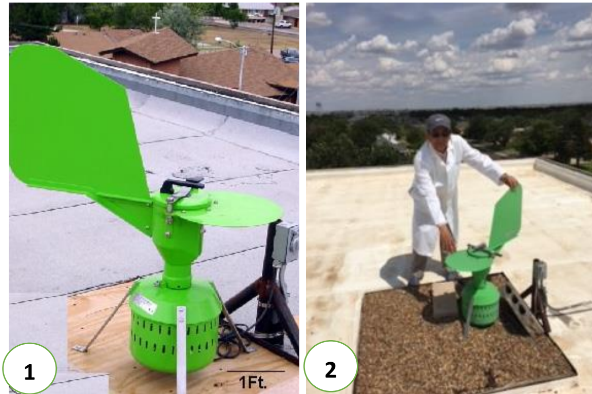
Figure 5-1: Burkard Volumetric Spore Trap on the roof top of NSB, at the West Texas A&M University, Canyon, Texas. Fig. 5-2: Researcher P. Banerjee working with the Burkard Volumetric Spore Trap.
