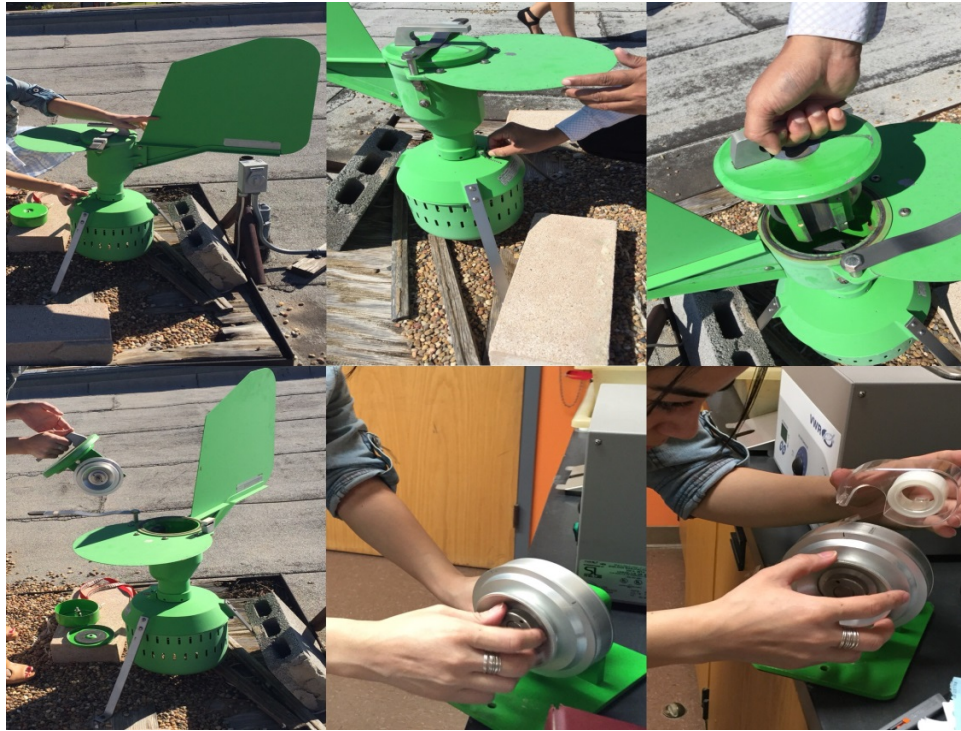
Figure 1. Steps in changing the Burkard spore trap
